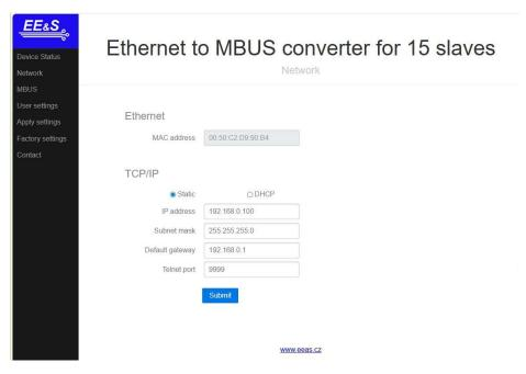
The MBUS interface setting is available under the **MBUS** panel on the left side. In the **Settings** section, the **TCP port** for the uplink communication as well
